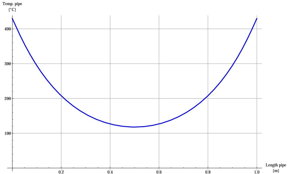
The temperature of pipe from calculation with assumption of constant temperature in cross section and no heat transfer in insulation in x - direction (red line) and from CFD results (blue line) are as below :
