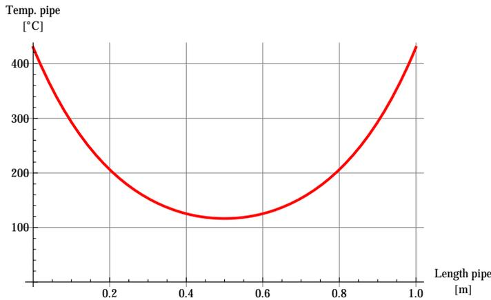
Heat flux on insulation external surface:  $q(x) = U_{ins} (T_m(x) - T_{air})$  :
