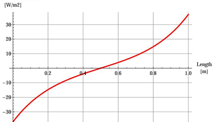
Conclusion: the x-direction heat flux through insulation is one order of magnitude smaller and, within reasonable approximation,  $dQ_{loss}$  travels only perpendicular on the x-direction and is constant in any cylindrical cross section.
