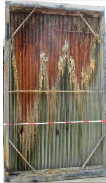
Corroded metallic air preheater
